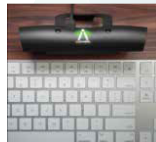
Green light = Disinfected
